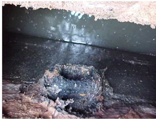
Photo #3 shows lateral pipes that have corroded completely shut
